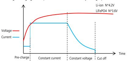
© 3 stage charging curve(Lead-Acid battery charger)
