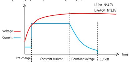
© 3stage charging curve(Lead-Acid battery charger)
