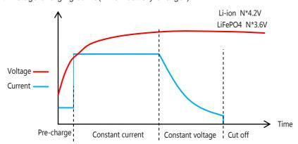
③ 3stage charging curve(Lead-Acid battery charger)
